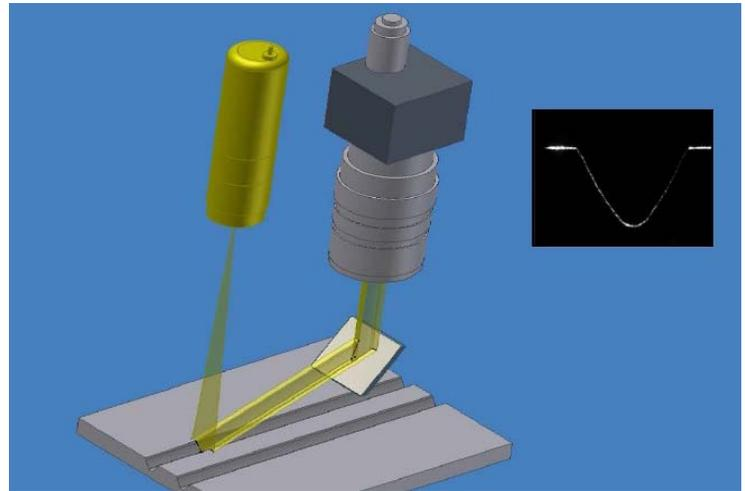
A precision laser laser-holographic module (yellow) projects onto the O-ring groove, whose shape is reflected towards a special TV camera that receives the contour of the groove in submillimetre detail.
